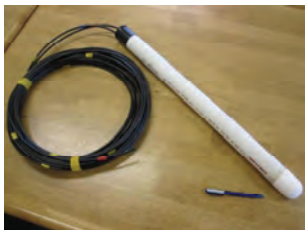
At most sites, 2-3 lysimeters are installed to account for spatial variability and to serve as back-up in the event of equipment failure.
