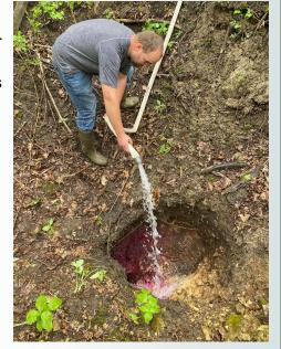
Dye tracing consists of installing charcoal dye receptors in various springs and other water sources in the study area, followed by pouring a unique, non-toxic, environmentally safe, fluorescent dye
